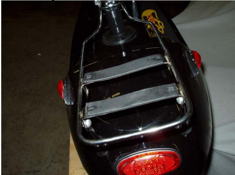
Then place the trunk on the rack over the rubber bushings. The two metal plates are placed inside the trunk and secured to the rack with the four enclosed screws and nuts.
