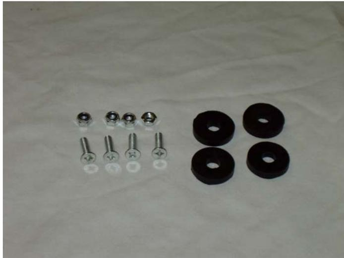
On the foot rest area of your scooter body are two holes on each side. Simply insert the bolt into the hole and place the rubber washer in-between the scooter body and metal frame underneath. Secure the body to the frame with the enclosed lock nuts. After your body is properly secured, attach the enclosed footpad decals to each side.
