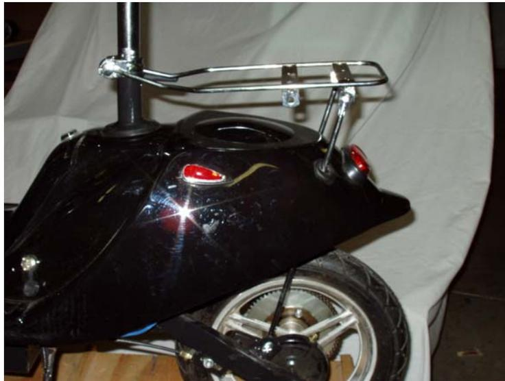
Attach the optional trunk to the trunk rack. Your trunk comes with the necessary hardware to attach the trunk to the rack if you choose. In the picture below are 2 rubber bushings and metal plates along with 4 screws and nuts.
