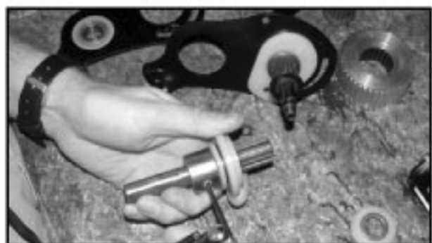
5. The three bolts and spacers that hold the centre section together can now be removed, allowing it to be stripped. We recommend removing the drive pulley on the lower main drive shaft before the centre section bolts are removed.
