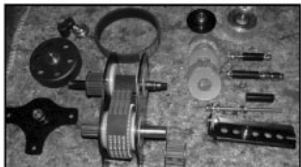
5. The three bolts and spacers that hold the centre section together can now be removed, allowing it to be stripped. We recommend removing the drive pulley on the lower main drive shaft before the centre section bolts are removed.
