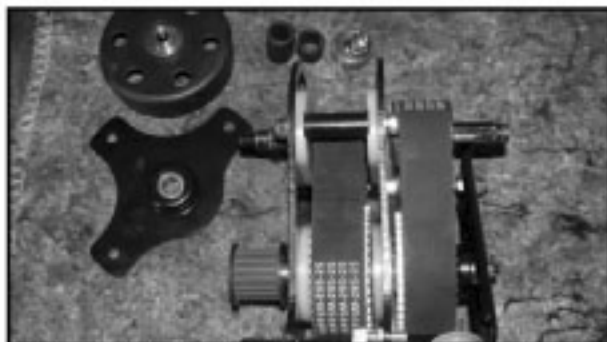
2. Remove the clutch drum, gearbox bracket, spacers and shaft bearing from the top shaft. To remove the clutch drum, it may be necessary to grip the shaft with a wrench. (Remove the long spacer on the shaft first to make room for the wrench.) The holes in the drum are there so a screwdriver may be placed through them for better grip.
