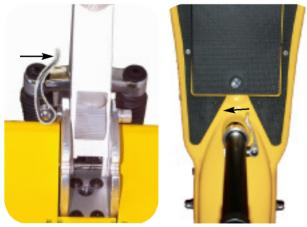
Securely tighten the folding mechanism quick release lever and the seat tube quick release lever. Remember to adjust the tensioner nuts if necessary.
