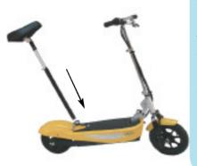
Fully insert the seat assembly and tighten the seat tube quick release lever at the base of the seat tube. Adjust seat height with supplied allen wrench. Do not adjust seat height at the base of the seat tube.
