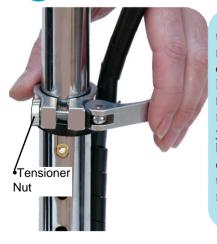
Tighten the quick release lever to lock the handlebars in place. You may need to adjust the tensioner nut on the quick release lever to hold the handlebar firmly in position. Check for proper tightness by holding the front wheel stationary inbetween your feet while wiggling the handlebars. If the handlebars are loose open the quick release lever, tighten the tensioner nut, close the quick release lever again and check again for tightness.
