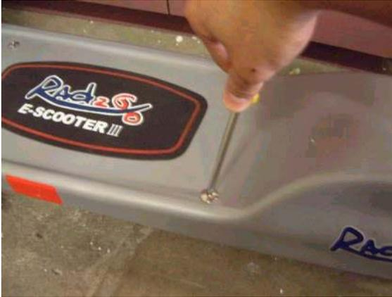
Step 1) Remove the 3 screws from the deck, use the Medium size Allen wrench to remove screws as shown in Figure 1. Lift the deck.
