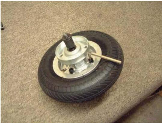
Step 6.) Remove the Allen bolts from the rim of the tire; you must first cut  $\frac{1}{2}$ " off of the medium size Allen wrench (use hack saw). The rim will split into 2 pieces. Once apart, replace the old tire with the brand new tire you have just received. Reassemble the rim back onto the tire.
