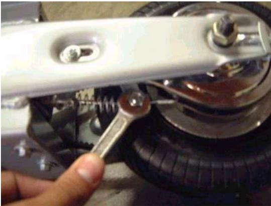
Step 4.) Loosen the brake adjustment bolt as seen in Fig 4. Do not completely remove this bolt. It should loosen to the point where the line traveling through the “brake spring” can be removed. Next remove the drive belt from the tire sprocket. Once this has been completed, the rear tire and hub can be removed from the scooter.
