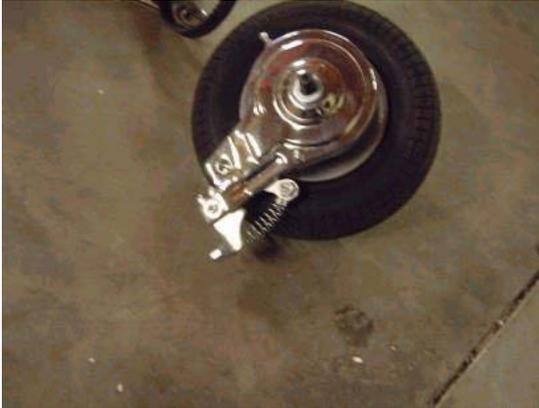
Step 9.) Insert the “L”-shaped bracket onto the brake shield. The hole for this bracket is located farthest from the wheel axle on the bracket itself. The bracket should be placed on the “tire-side” of the shield (as opposed to the outer side). (Wheel shown as removed to better display “L”-shaped bracket). Next, place the brake spring back into its original setting as seen in Fig 9.
