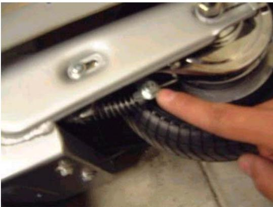
Step 10.) Insert the brake line through the “L”-shaped bracket and through to the brake adjustment bolt (as seen in Fig 10). Pull the line tighter to get a “stiffer” brake response. Please test the brake at low speeds before using. If your brakes are too tight, loosen the adjustment bolt once again and adjust the brake wire accordingly. Use the 4 Phillips screws to bolt down the scooter’s deck. You have now successfully replaced your scooter’s rear tire!
