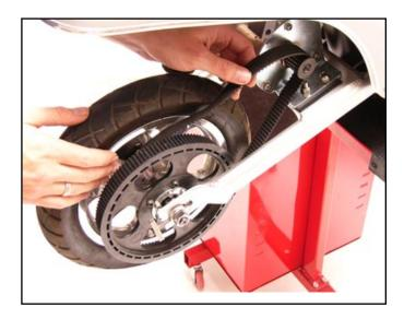
6. Slide belt off the rear pulley toward the wheel.
