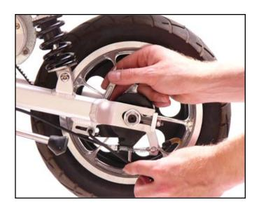
4. Loosen and remove the brake arm bolt using a 4mm allen wrench and an 8mm wrench.steps are not necessary to remove
