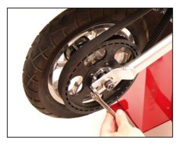
5. Loosen each tensioner nuts several turns and move the rear wheel forward to detention drive belt.
