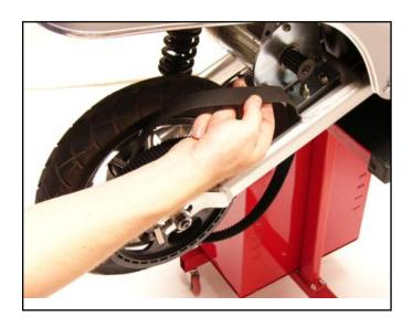
7. Pull the belt off of the motor sprocket.
