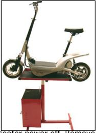
1. Turn scooter power off. Remove both batteries and place the scooter on a sturdy stand or otherwise elevate the rear wheel.
