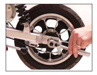
3. Loosen both 19mm axle nuts.
