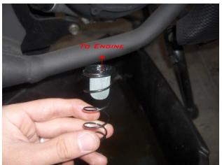
Let the motor oil drain until only a few drops fall every few seconds. Put the *cleaned* Oil Filter and the spring back into the engine as shown to the left. If done incorrectly, the filter will not be efficient in collecting dirt and sludge from the engine.
