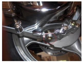
With the bike on its center stand, locate the Gear Oil Drain Plug that is under the rear of the drive belt case. Remove it with a 10mm socket or wrench.
