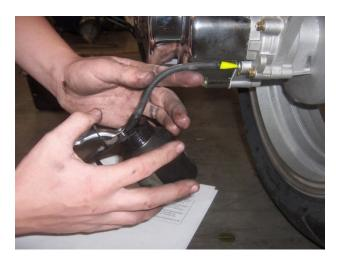
Fill a pistol grip oil can with 0.10L of 80W-90 Gear Oil. If it has been cold and you find that the transmission is not as smooth as normal, use lighter 75 weight gear oil.
