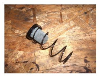
A small spring and Screen Type Oil Filter will also pop out. Place these two items off to the side and wash them clean by flushing them with new 10W-40 motor oil.
