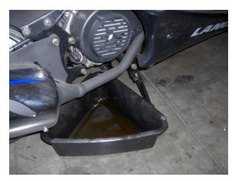
Place a drain pan under the Drain Plug and remove the plug with a 17mm socket or wrench.
