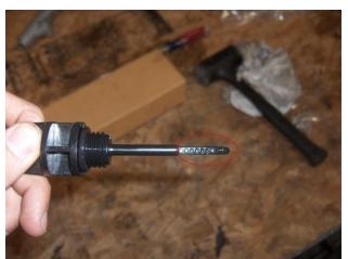
Check the oil with the dipstick. Place the dipstick in the motor but do not screw it in. Pull it out and make sure that the oil reading is within the hash-marks, then add or drain oil accordingly until it is.
