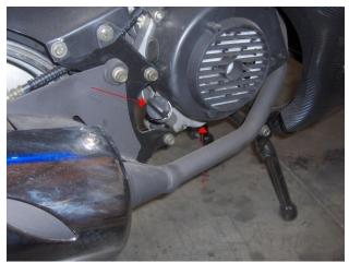
The Drain Plug and the Dipstick for the motor oil are located on the right side of the bike.
