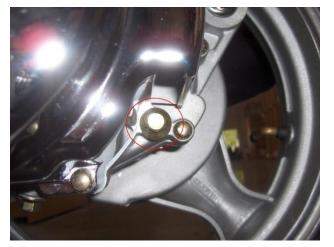
Unscrew the fill bolt (pictured to the left) with a 10mm socket or wrench.
