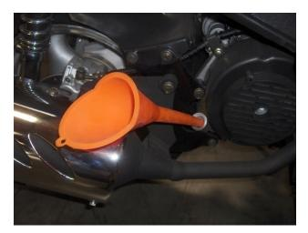
Using a funnel, pour 0.75 quarts of 10W-40 Motor Oil into the engine.
