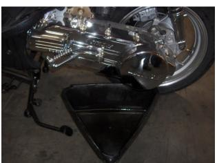
Once all the oil has drained out, replace the drain bolt using a torque wrench set at 20 lbs/ft.
